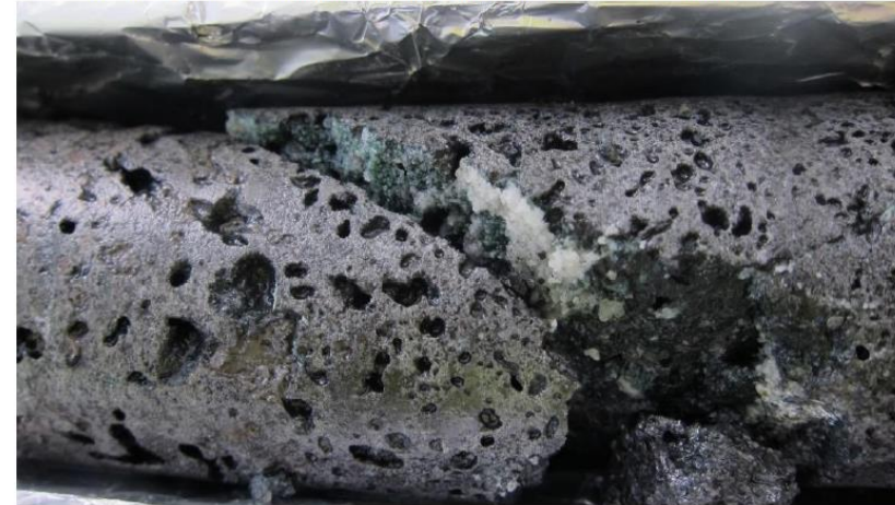
EXHIBIT 21: Rock core from the Carbfix project in Iceland shows carbonates created from injected CO 2
