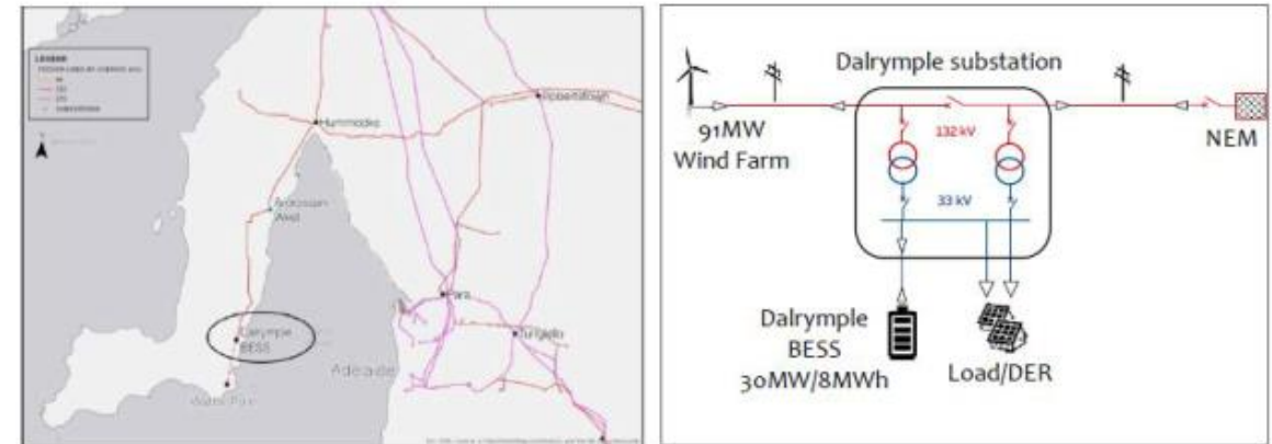
Figure 15 ESCRI battery network location – a simple network diagram
